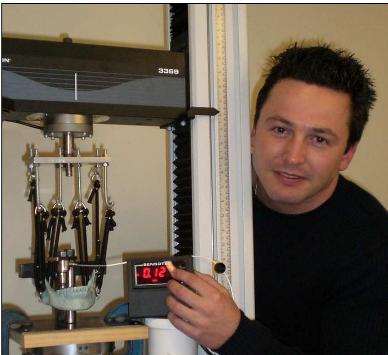
Figure 2. Markus Perchtaler alongside the mandible test rig. The image shows an adjustable position load cell (can be swung in an arch to any tooth position) placed over the first molar. Elastic muscles attached to the muscle attachment points and pull hooks attached to the universal testing machine load cell enable the recording of the bite force on the teeth and amount of muscle force required to achieve this.
