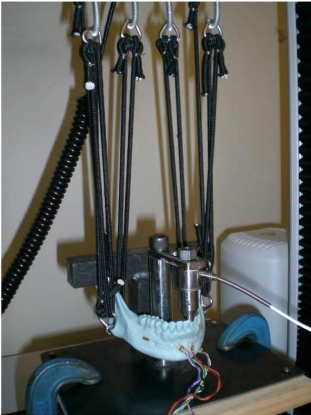
Figure 4. Mandible in loaded from the Masseter, Temporalis and Medial Pterygoid muscle groups. Strain gauges attached to the buccal and lingual of the mandible below the first molar position on both the working and balancing side. Load cell is positioned to record the bite force at the central incisor position.
