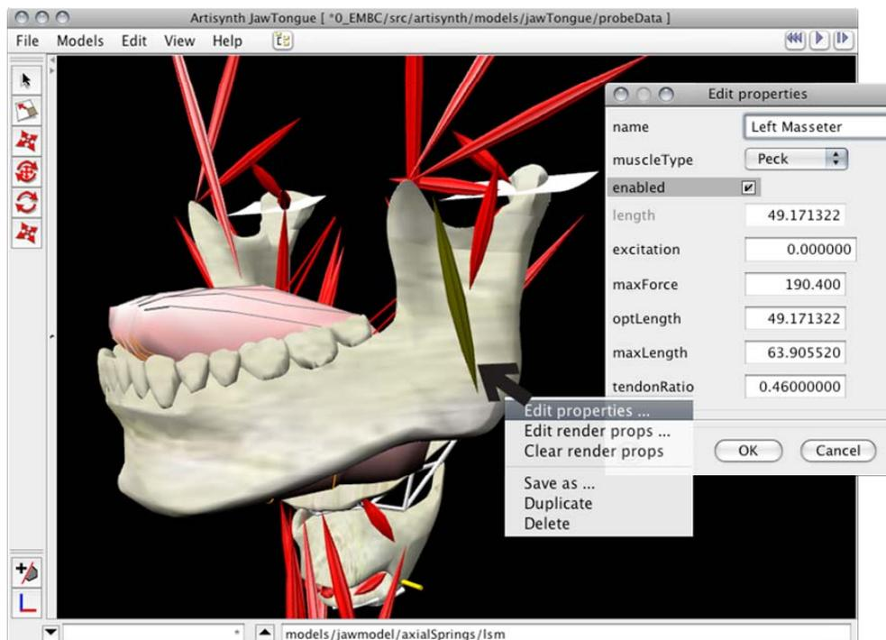
Figure 1: The dynamic Jaw-Tongue-Hyoid model in ArtiSynth with a property-editing panel for the selected jaw muscle. (Figure is from a artisynt model, courtesy of Ian Stavness)
