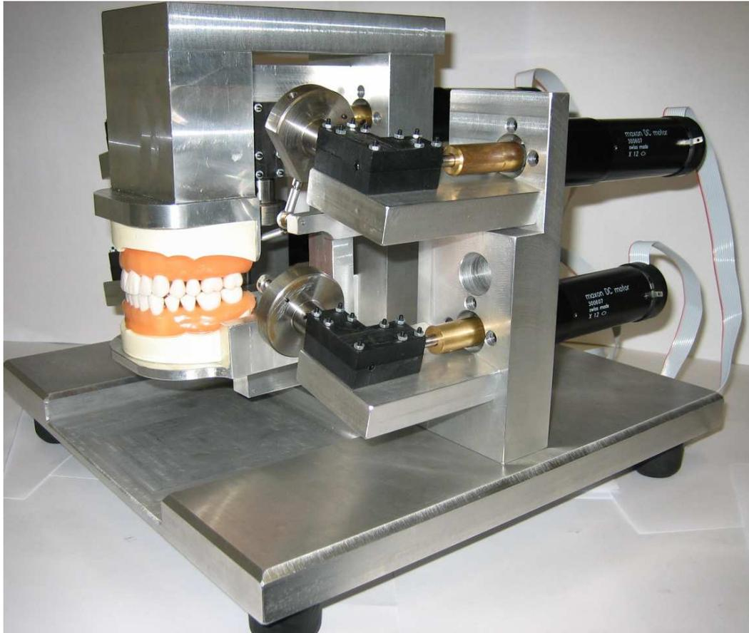
*Figure 1* Physical model of the chewing robot.
