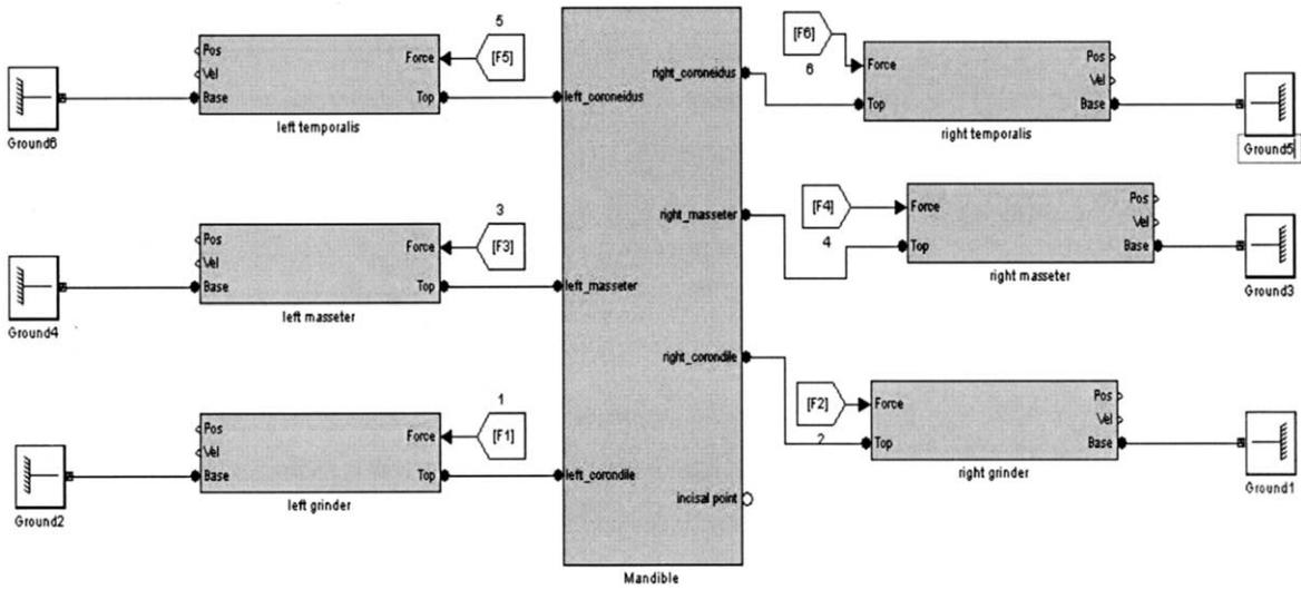
Fig. 5. Screenshot of the jaw mechanism in SimMechanics. The middle block stands for the mandible, the most left and right blocks for the ground and the blocks between the mandible and ground for muscular actuators.
