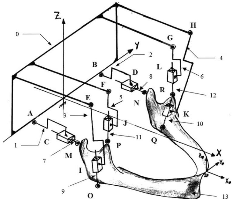
Fig. 4. A kinematic sketch of jaw mechanism. Letters C, D, I, J, K, L stand for muscular actuators, the numbers for links making up the mechanism and the remaining letters for actuators ground and mandible attaching points (or spherical joints).
