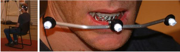
**Figure 1:** Left: Set-up of the experiments with 6 markers (3 at a head band and 3 on a custom-made brace). Right: Enlarged view of the custom-made brace.
